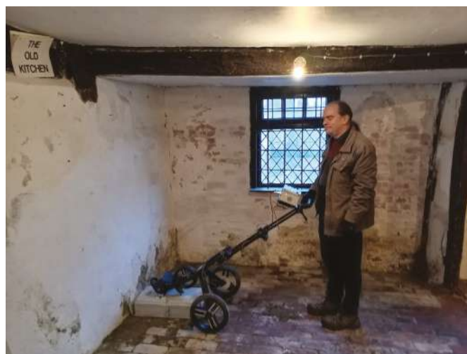
Ground Radar Survey in the Tudor Kitchen, 9th December 2023. Photograph by Dr. Alan Starr
